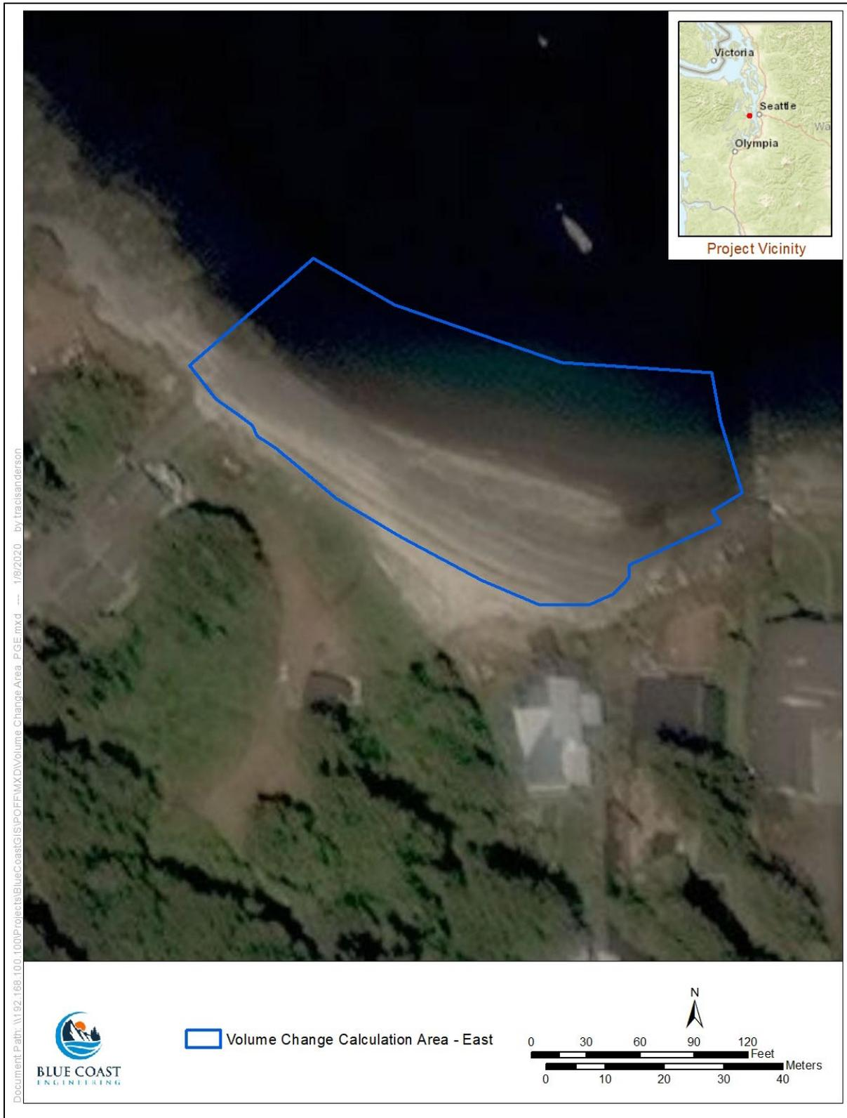
**Figure 13. Area of Point Glover east where volume changes were calculated.**
