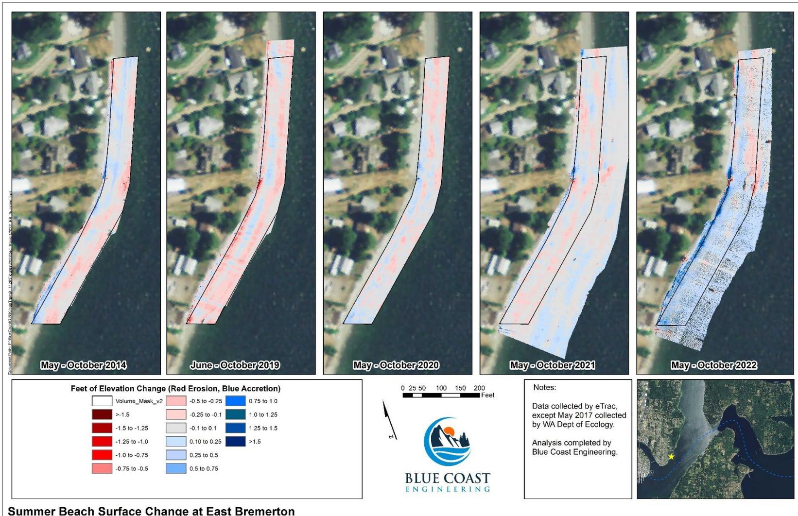
Figure 5. East Bremerton summer elevation change in 2014, 2019, 2020, 2021, and 2022.
