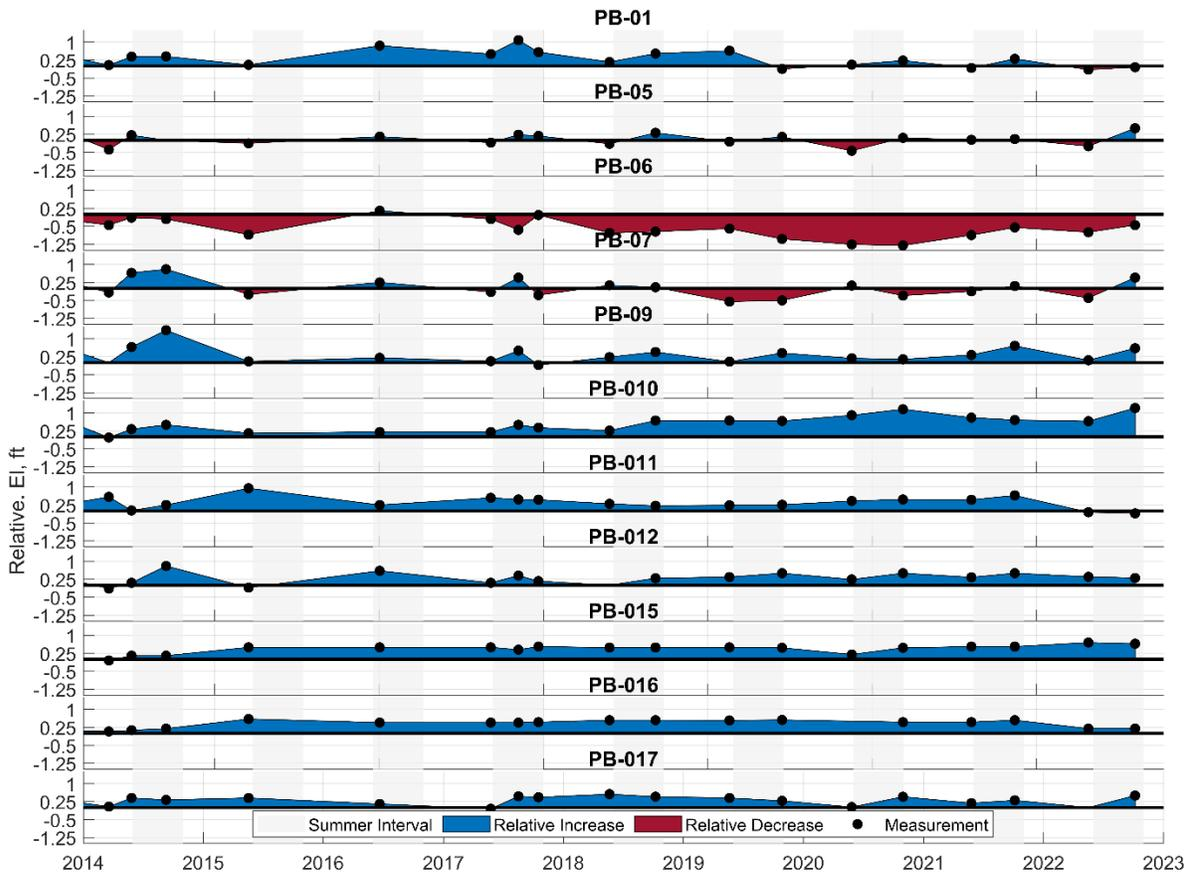
**Figure 6. Time series of relative beach elevation from 2014 through 2022 at all beach photo survey sites along Pleasant Beach. Blue indicates accretion relative to the 2005 starting point and red indicates erosion relative to the 2005 starting point.**
