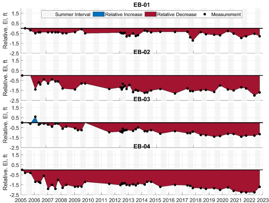
**Figure 3. Time series of relative beach elevation from 2005 through 2022 at beach photo survey sites EB\_01 to EB\_04. Blue indicates accretion relative to the 2005 starting point and red indicates erosion relative to the 2005 starting point.**
