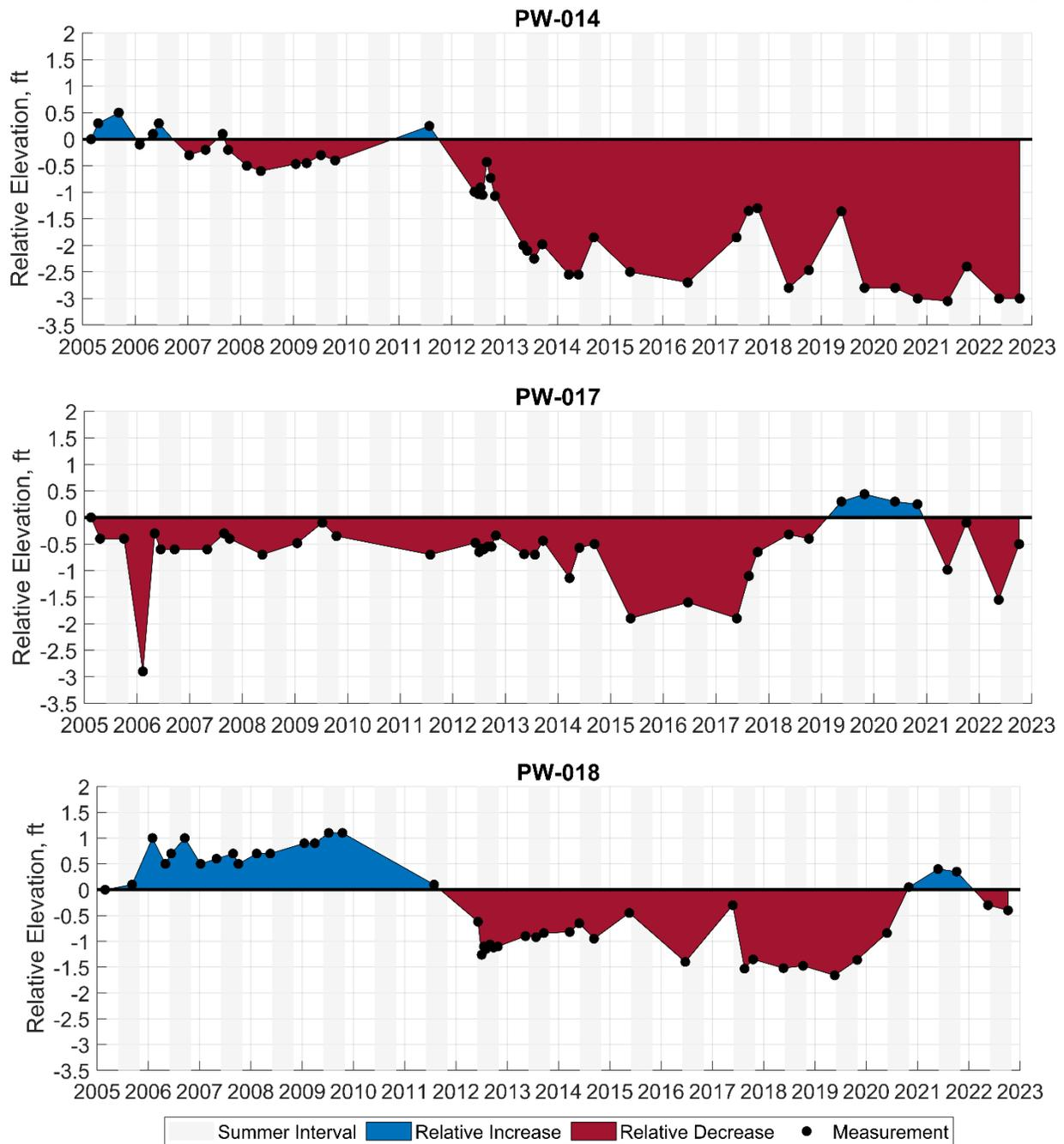
**Figure 17. Time series of relative beach elevation from 2005 through 2021 at beach photo survey sites PW\_14 and PW\_18. Blue indicates accretion relative to the 2005 starting point and red indicates erosion relative to the 2005 starting point.**
