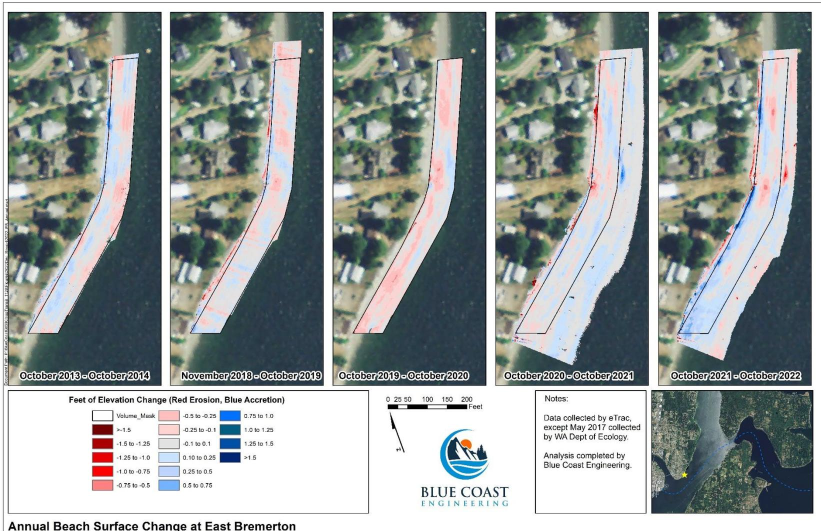
Figure 4. East Bremerton annual elevation change from 2013 to 2014, from 2018 to 2019, 2019 to 2020, 2020 to 2021, and 2021 to 2022.
