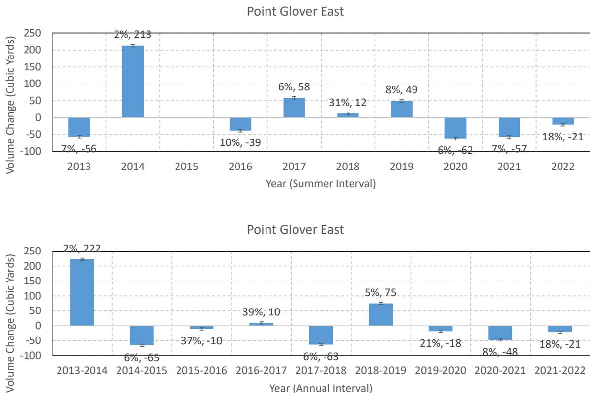
**Figure 14. Volume change (cubic yards, CY) in calculation area at Point Glover East. The volume change (CY) and error as a percentage of the total change are shown for each measurement.**
