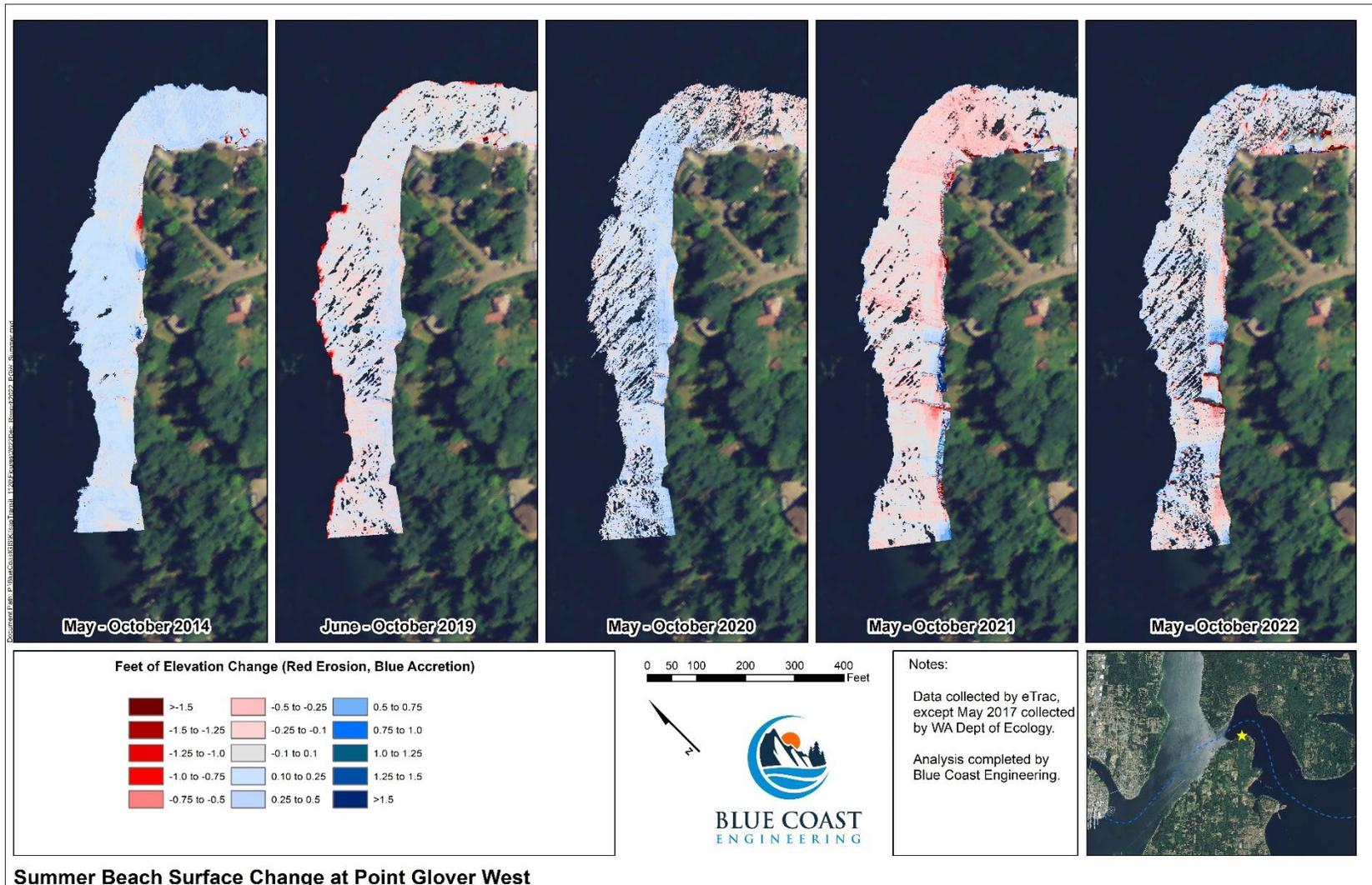
Figure 10. Point Glover West summer elevation change in 2014, 2019, 2020, 2021, and 2022.
