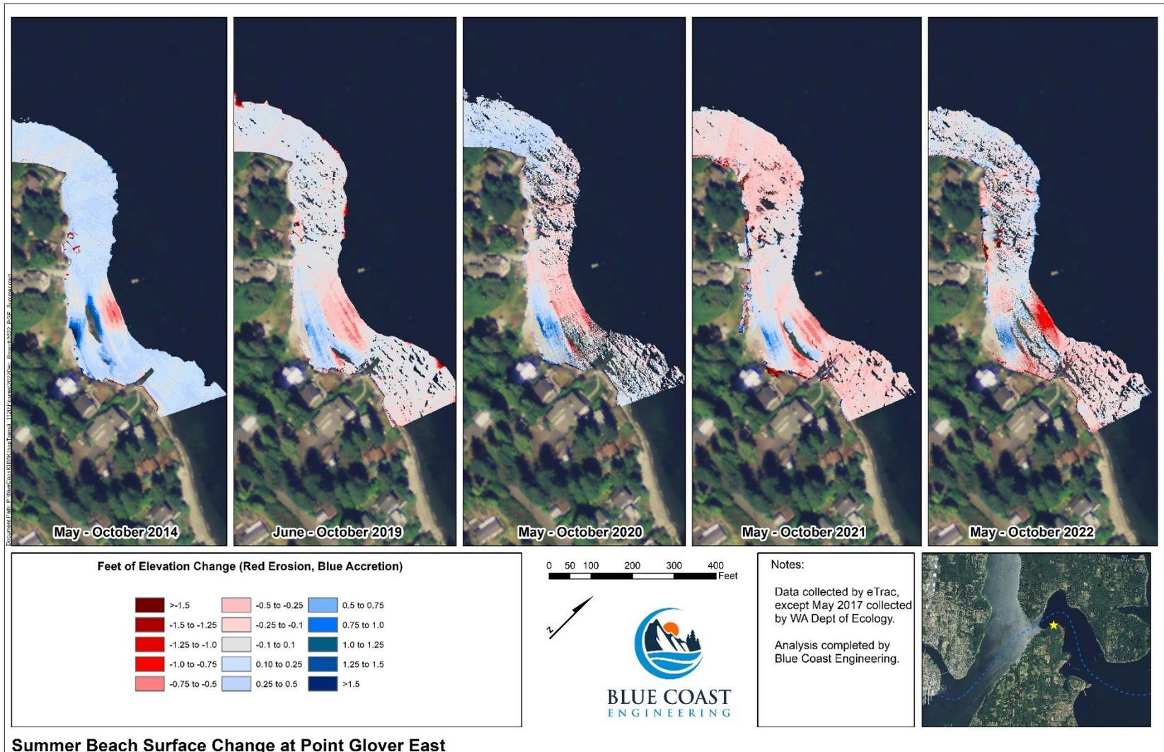
Figure 12. Point Glover East summer elevation change in 2014, 2019, 2020, 2021, and 2022.
