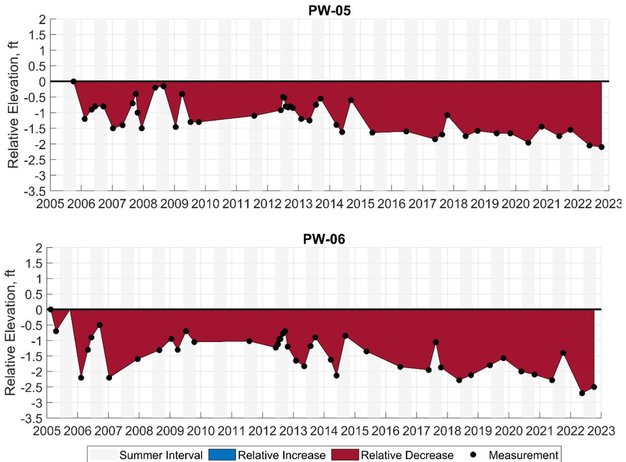
**Figure 16. Time series of relative beach elevation from 2005 through 2022 at beach photo survey sites PW\_05 and PW\_06. Blue indicates accretion relative to the 2005 starting point and red indicates erosion relative to the 2005 starting point.**
