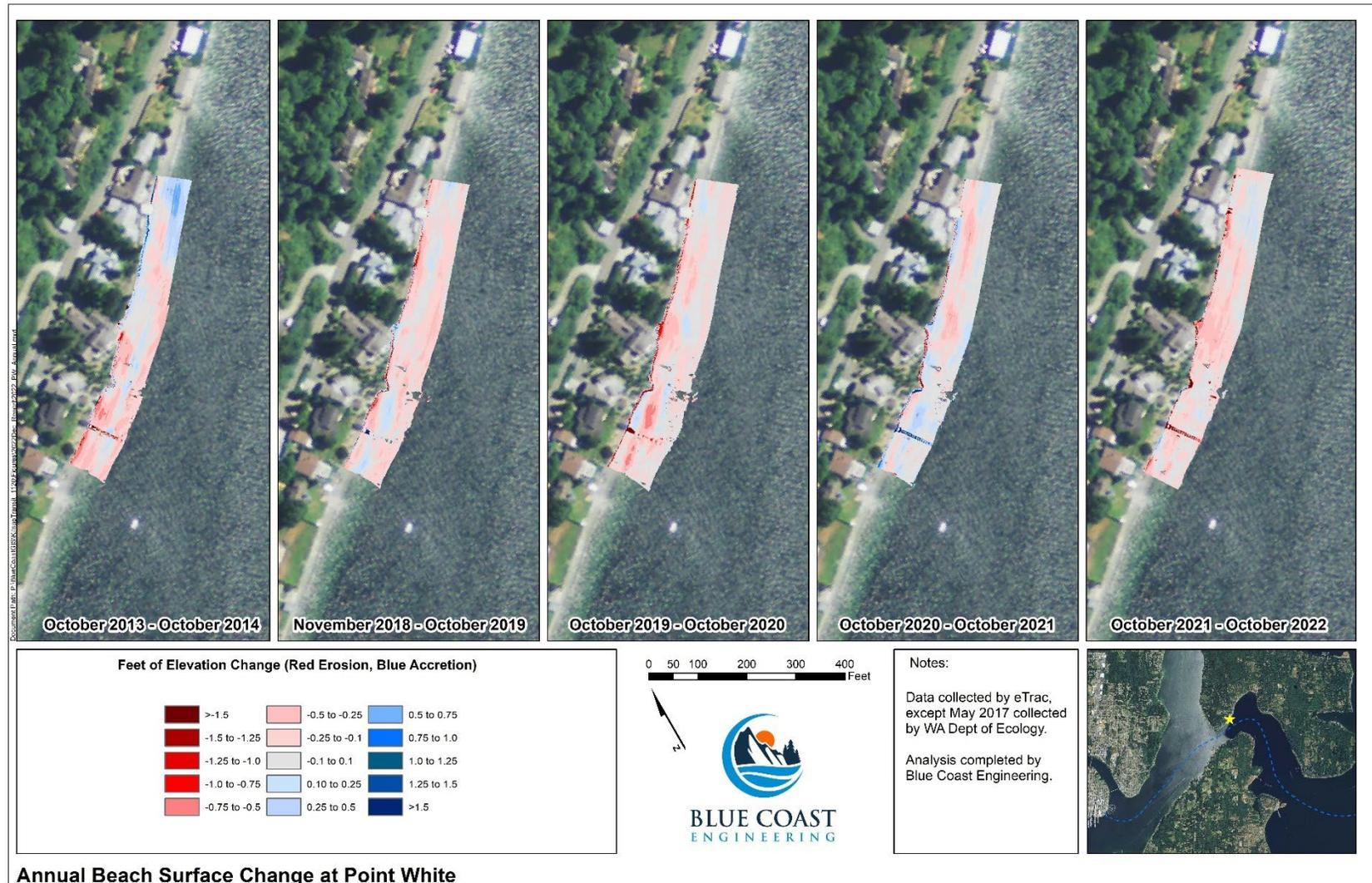
Figure 18. Point White elevation change over four 1-year intervals from 2013 to 2022.
