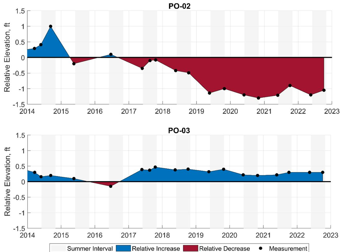
**Figure 15. Time series of relative beach elevation from 2014 through 2022 at beach photo survey sites PO\_02 and PO\_03. Blue indicates accretion relative to the 2005 starting point and red indicates erosion relative to the 2005 starting point.**
