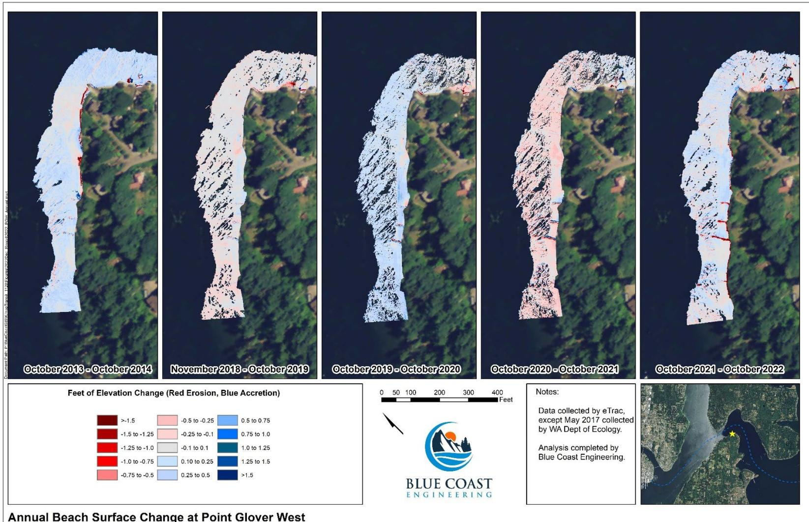
Figure 9. Point Glover West elevation change over five 1-year intervals from 2013 to 2022.
