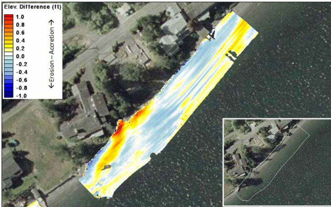
Figure 4-16: Elevation difference at Point White – Site 3 between 04 June and 12 November 2012
