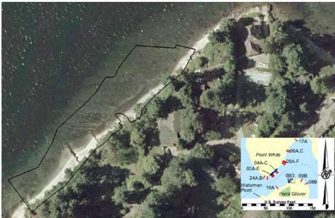
Figure 2-12: Volume calculation mask boundary for Point Glover – Site 9
