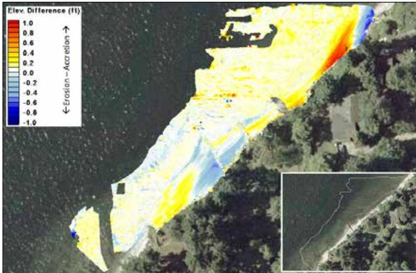
Figure 4-25: Elevation difference at Point Glover – Site 9 between 05 June 2012 and 13 November 2012
