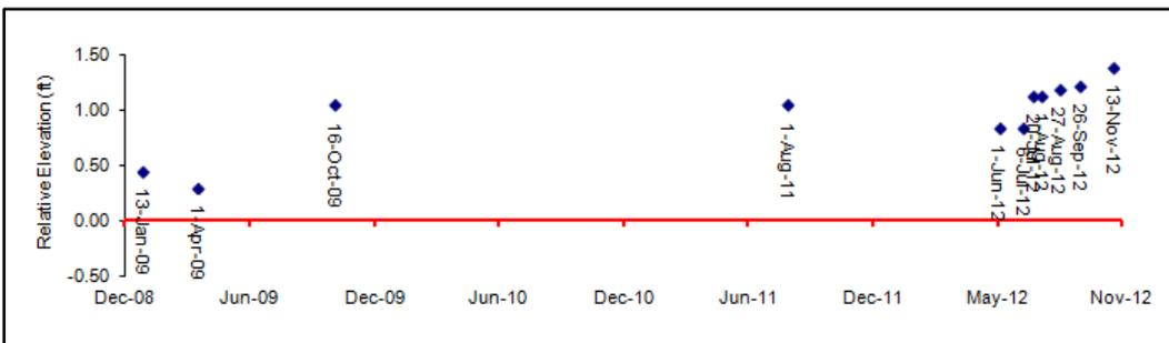
**Figure 4-34: Beach elevation measured at the toe of the bulkhead from January 2009 to November 2012 relative to February 2005 at Site EB\_16 on the southern end of East Bremerton**
