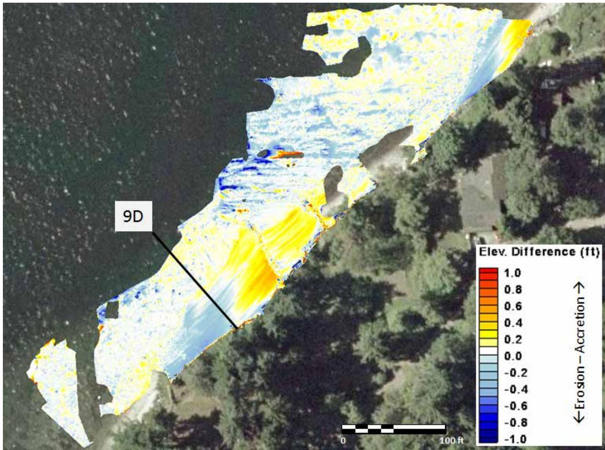
Figure 3-10: Difference map of laser scanning surveys measured at Site 9 on Point Glover between 8 September 2011 and 5 June 2012
