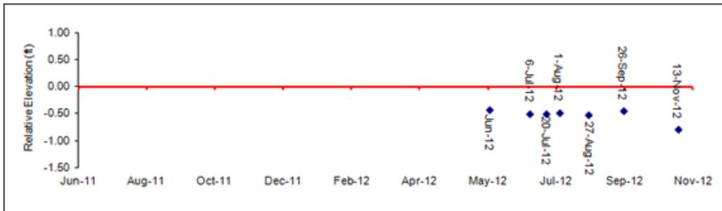
**Figure 4-33: Beach elevation measured at the toe of the bulkhead relative to February 2005 at Site EB\_01 on the southern end of East Bremerton**
