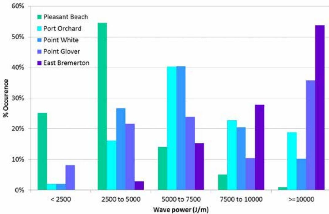
Figure 4-6: Histogram of wave power from RP1 measured along each shoreline
