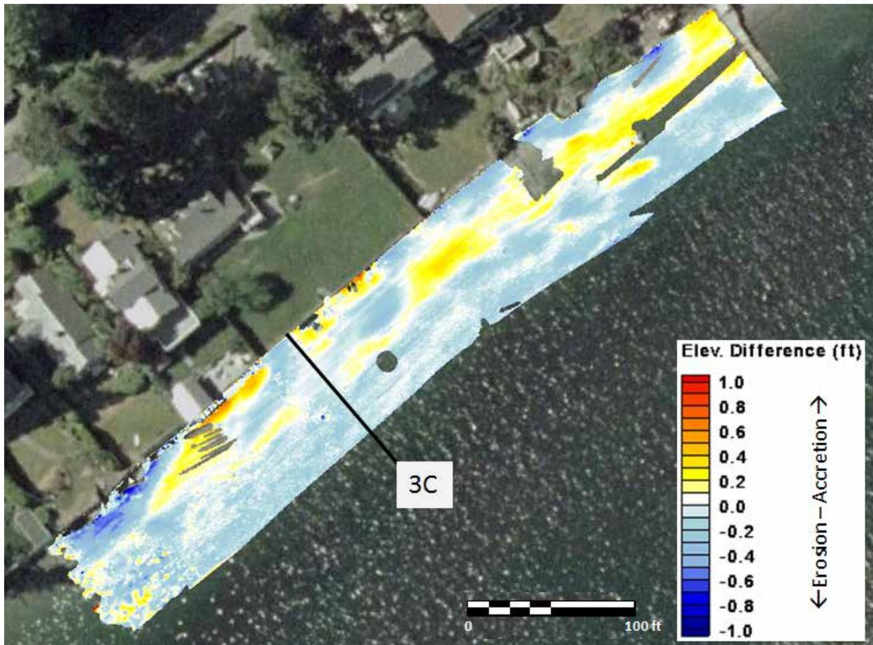
Figure 3-5: Difference map of laser scanning surveys measured at Site 3 on Point White between 9 September 2011 and 4 June 2012
