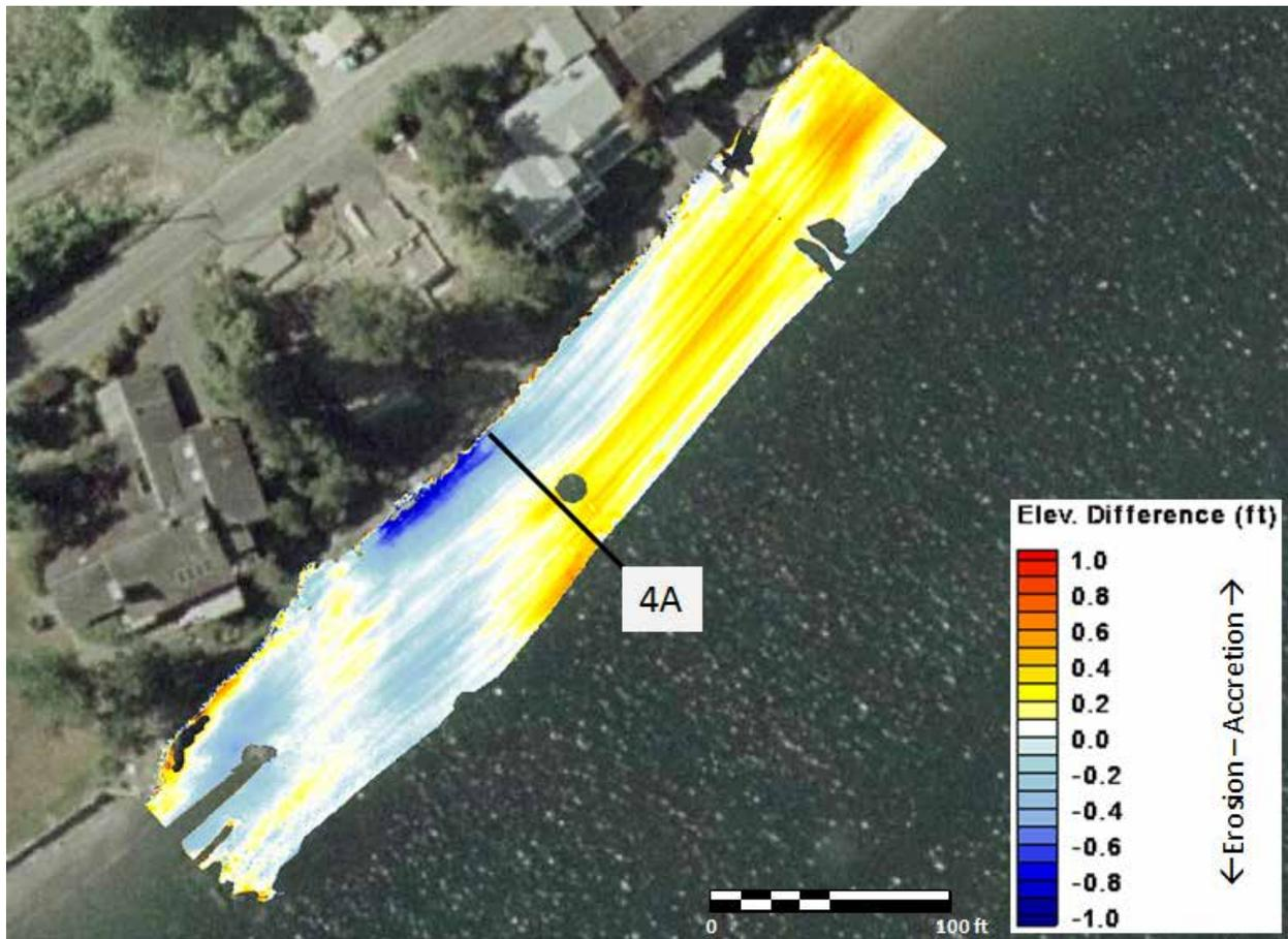
**Figure 3-6: Difference map of laser scanning surveys measured at Site 4 on Point White between 9 September 2011 and 4 June 2012**
