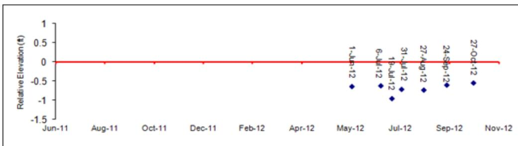
Figure 4-39: Beach elevation measured in June to October 2012 at the toe of the bulkhead relative to February 2005 at Site PG\_07 on Point Glover
