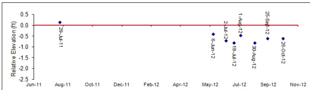
Figure 4-37: Beach elevation measured July 2011 to October 2012 at the toe of the bulkhead relative to February 2005 at Site PW\_11 on Point White
