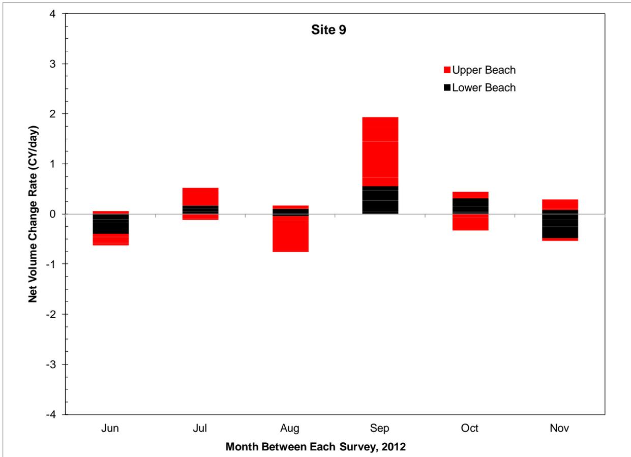
Figure 4-31: Calculated rates of volume change at Site 9 for each approximately month-long survey span during the Summer through Fall 2012 operations
