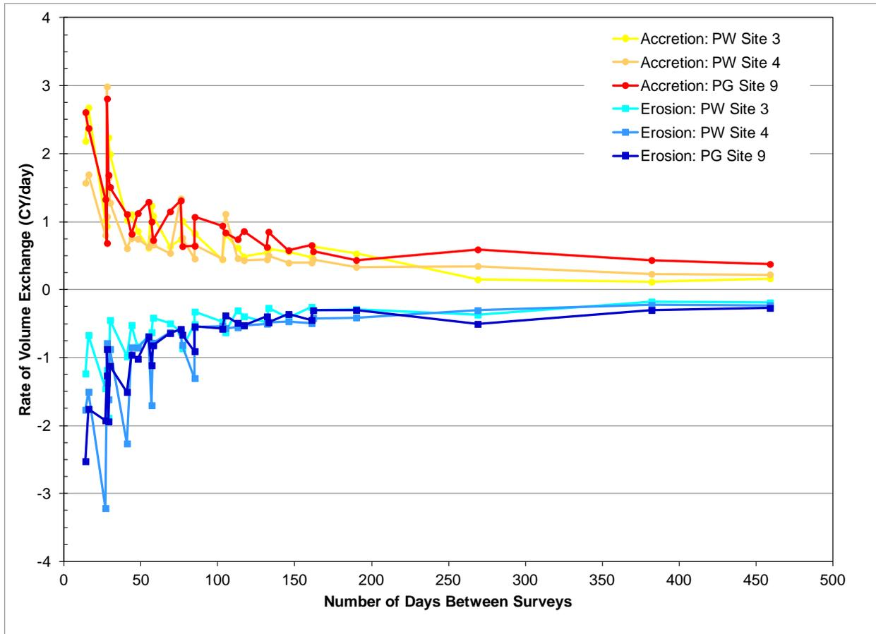
Figure 4-27: Calculated rates of erosion (negative volume; cooler color lines) and accretion (positive volume; warmer color lines) at each site for every survey period
