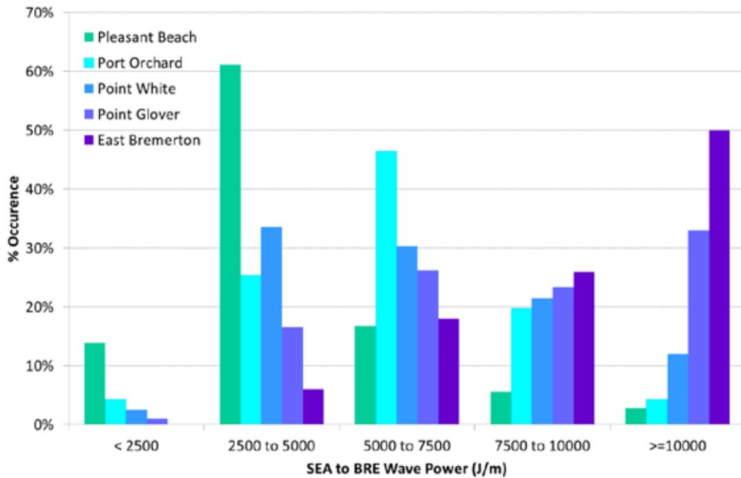
Figure 4-8: Histogram of wave power from RP1 while operating Seattle to Bremerton of RP1 measured along each shoreline
