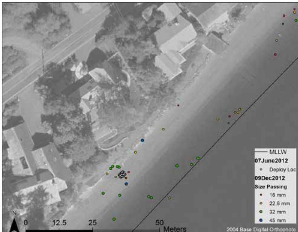
Figure 4-19: Tracer Locations from first to last survey dates at Site 4
