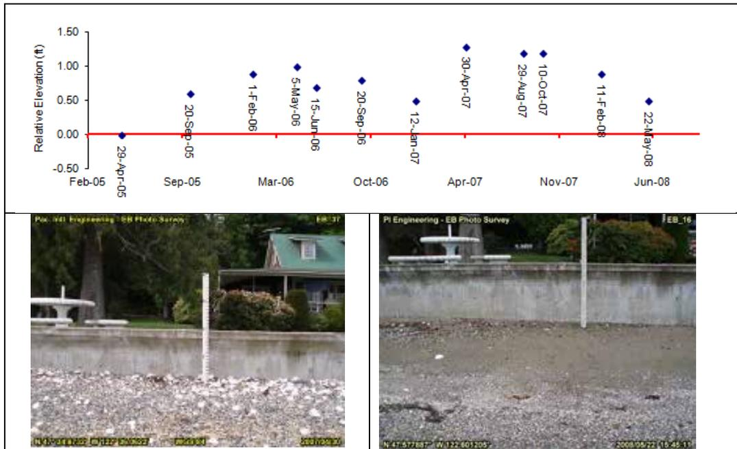
Figure 4-35: Beach elevation measured at the toe of the bulkhead from April 2005 to May 2008 relative to February 2005 at Site EB\_16 on East Bremerton; Photograph of Site EB\_16 on 29 April 2005 (bottom left) and photograph of Site EB\_16 on 22 May 2008
