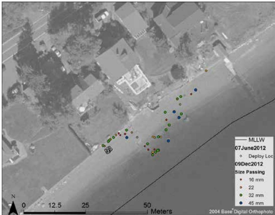
Figure 4-18: Tracer locations from first to last survey dates at Site 3
