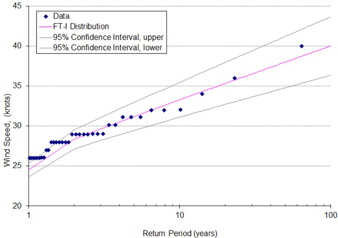
Figure 2-4: Wind speed as a function of return period for a FT-1 distribution
