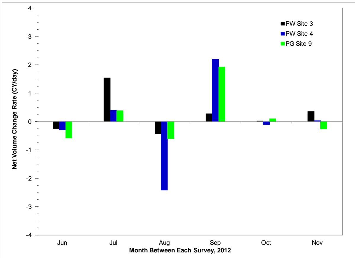
**Figure 4-32: Calculated rates of volume change at all sites for each approximately month-long survey span during the Summer through Fall 2012 operations**
