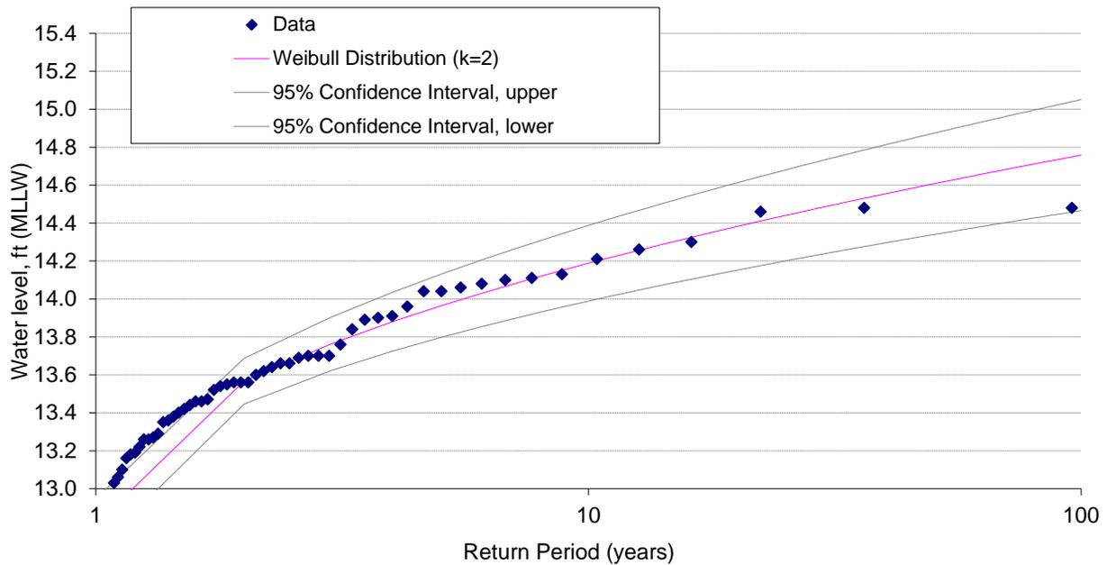
Figure 2-14: Water level as a function of return period for Weibull Distribution (k=2.00)
