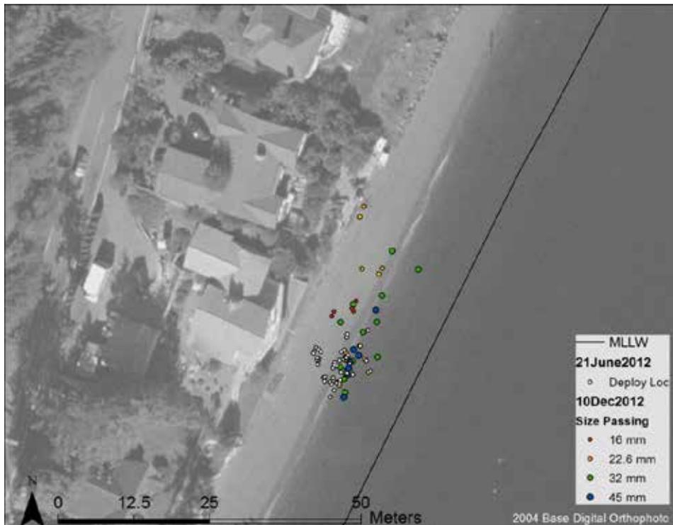
**Figure 4-20: Tracer Locations from first to last survey dates at Site 5**
