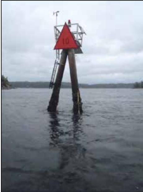
**Figure 2-5: Navigation aid at Point White with anemometer installed**
