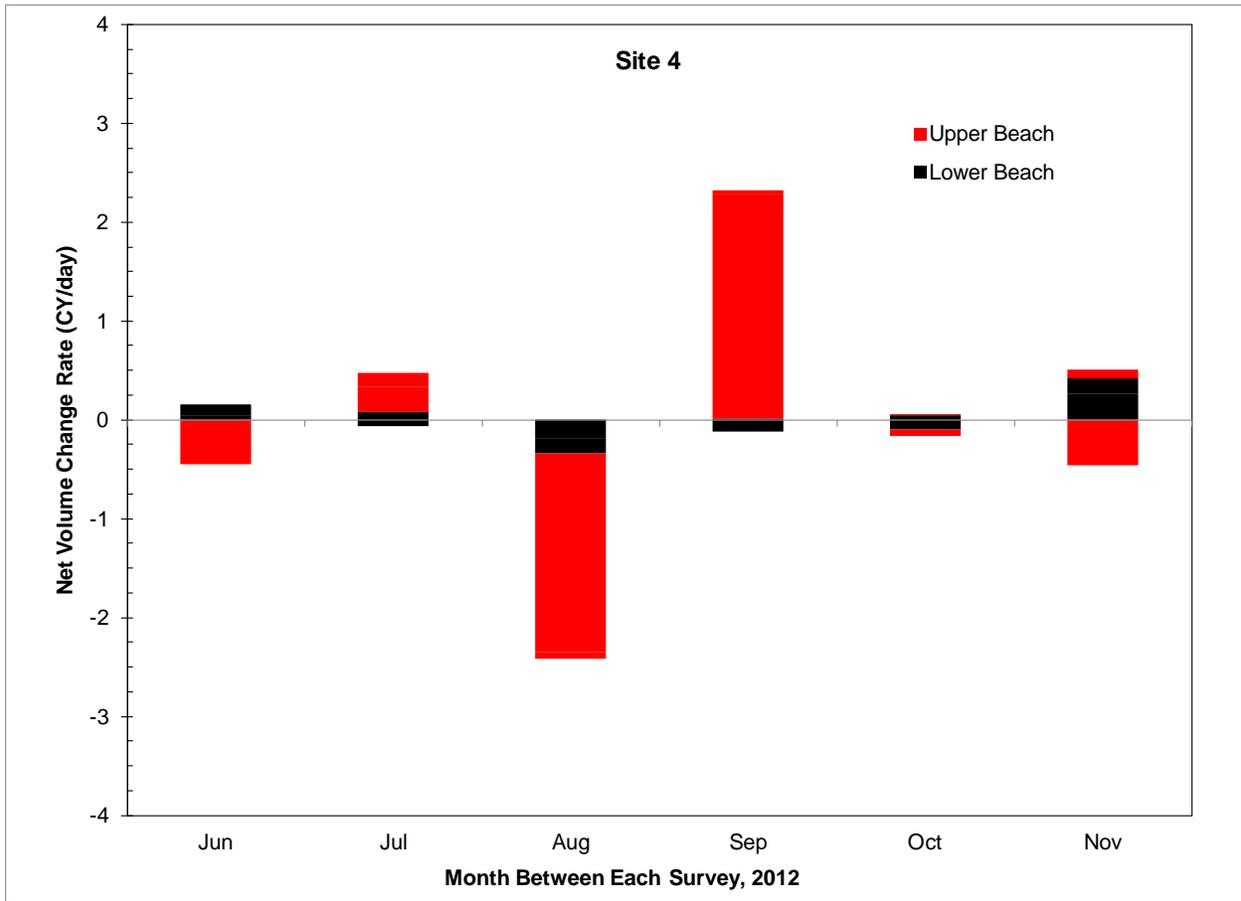
Figure 4-30: Calculated rates of volume change at Site 4 for each approximately month-long survey span during the Summer through Fall 2012 operations
