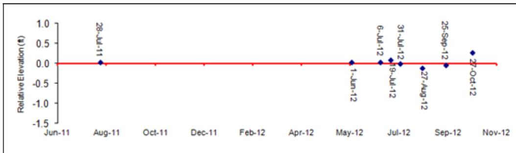
Figure 4-38: Beach elevation measured July 2011 to October 2012 at the toe of the bulkhead relative to February 2005 at Site PO\_02 on Port Orchard
