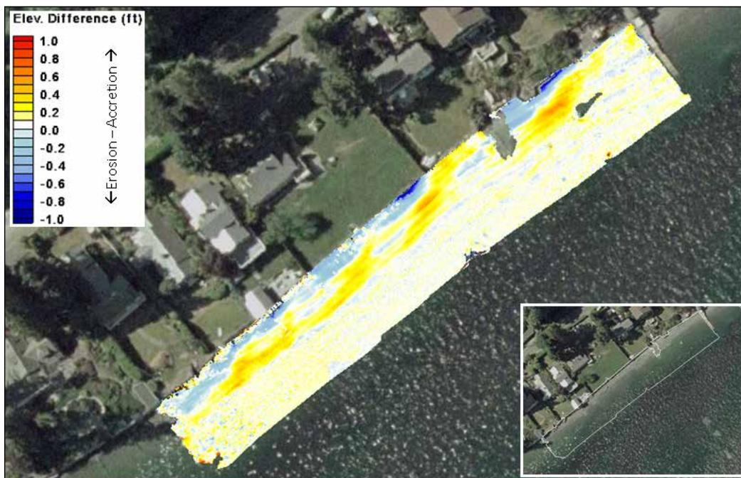
Figure 4-15: Elevation difference at Point White – Site 3 between 12 November 2012 and 11 December 2012
