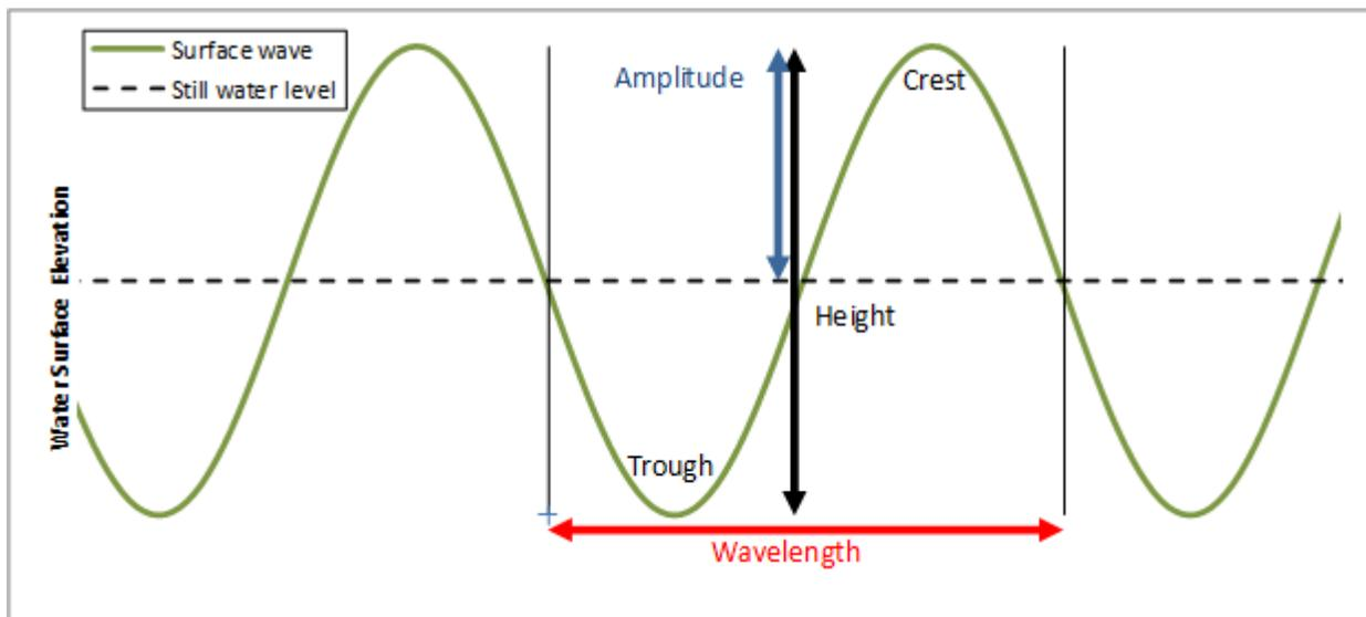
**Figure 2-8: Plot of idealized surface wave with wave properties defined**
