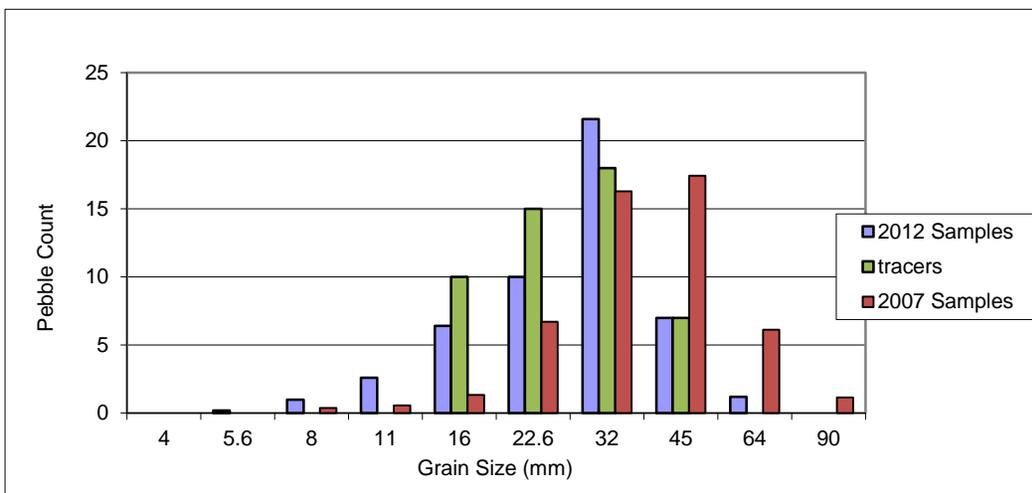
Figure 4-23: Comparison of the normalized frequency of the 2012 and 2007 beach samples and tracer sediments at Site 3 at 2' to 8.5' MLLW
