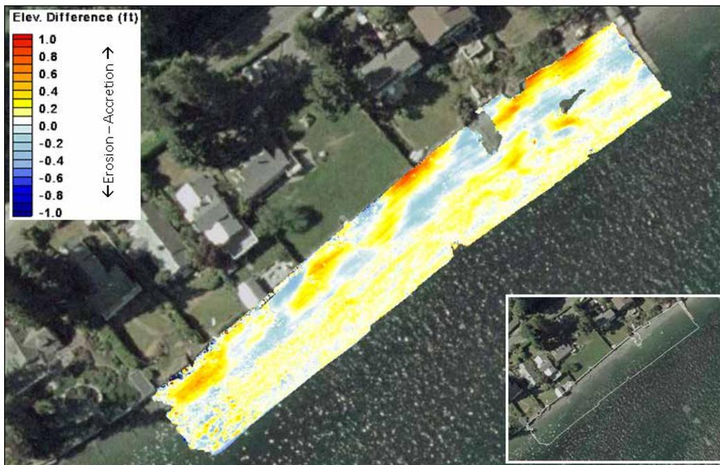
Figure 4-14: Elevation difference at Point White – Site 3 between 04 June 2012 and 12 November 2012
