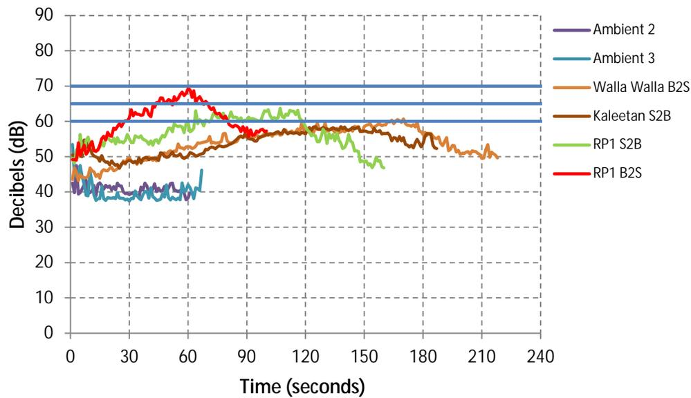
**Figure 4-46: Measurements of noise levels near Site 3 (Point White) for various vessels and ambient conditions in Rich Passage on 26 June 2012**
