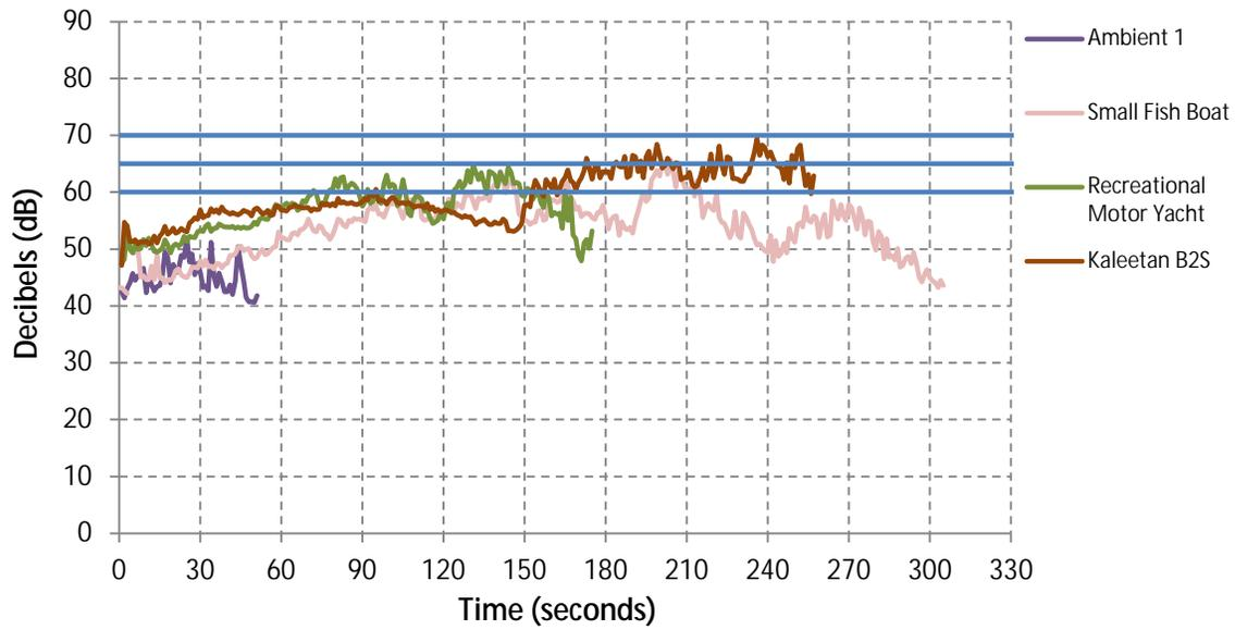
**Figure 3-12: Measurements of noise levels near Site 8 (Point Glover) for various vessels and ambient conditions in Rich Passage on 26 June 2012**
