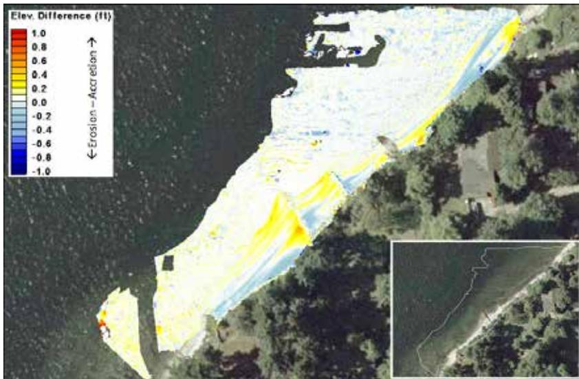
Figure 4-26: Elevation difference at Point Glover – Site 9 between 13 November 2012 and 13 December 2012
