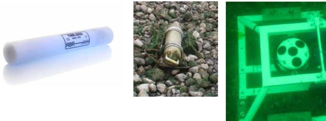
**Figure 2-7: RBR Wave and Tide Recorder (left), Coastal Leasing MacroWave (center), and Nortek AWAC (right)**
