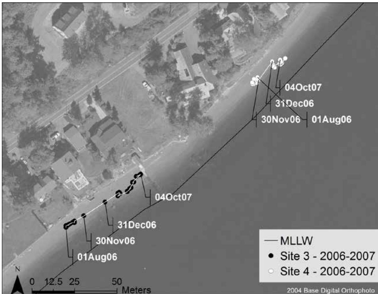
Figure 3-7: Location of tracer centroids for the 2006-2007 survey at sites 3 and 4
