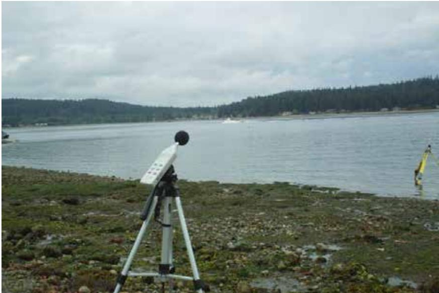
**Figure 2-15: Noise recording device located on Point Glover beach**
