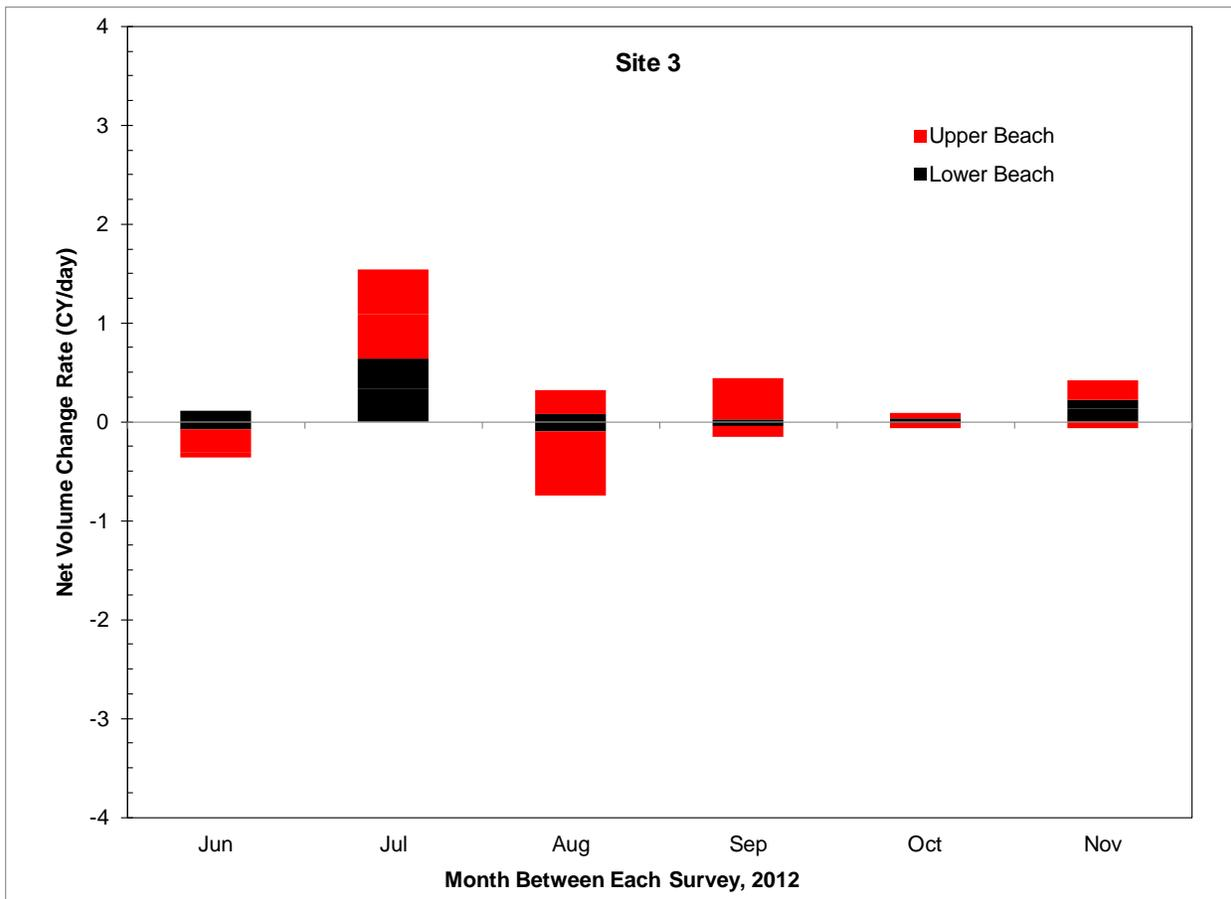
Figure 4-29: Calculated rates of volume change at Site 3 for each approximately month-long survey span during the Summer through Fall 2012 operations
