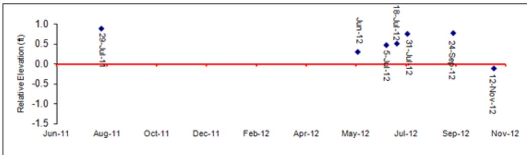
Figure 4-36: Beach elevation measured July 2011 to November 2012 at the toe of the bulkhead relative to February 2005 at Site PB\_07 on the Pleasant Beach
