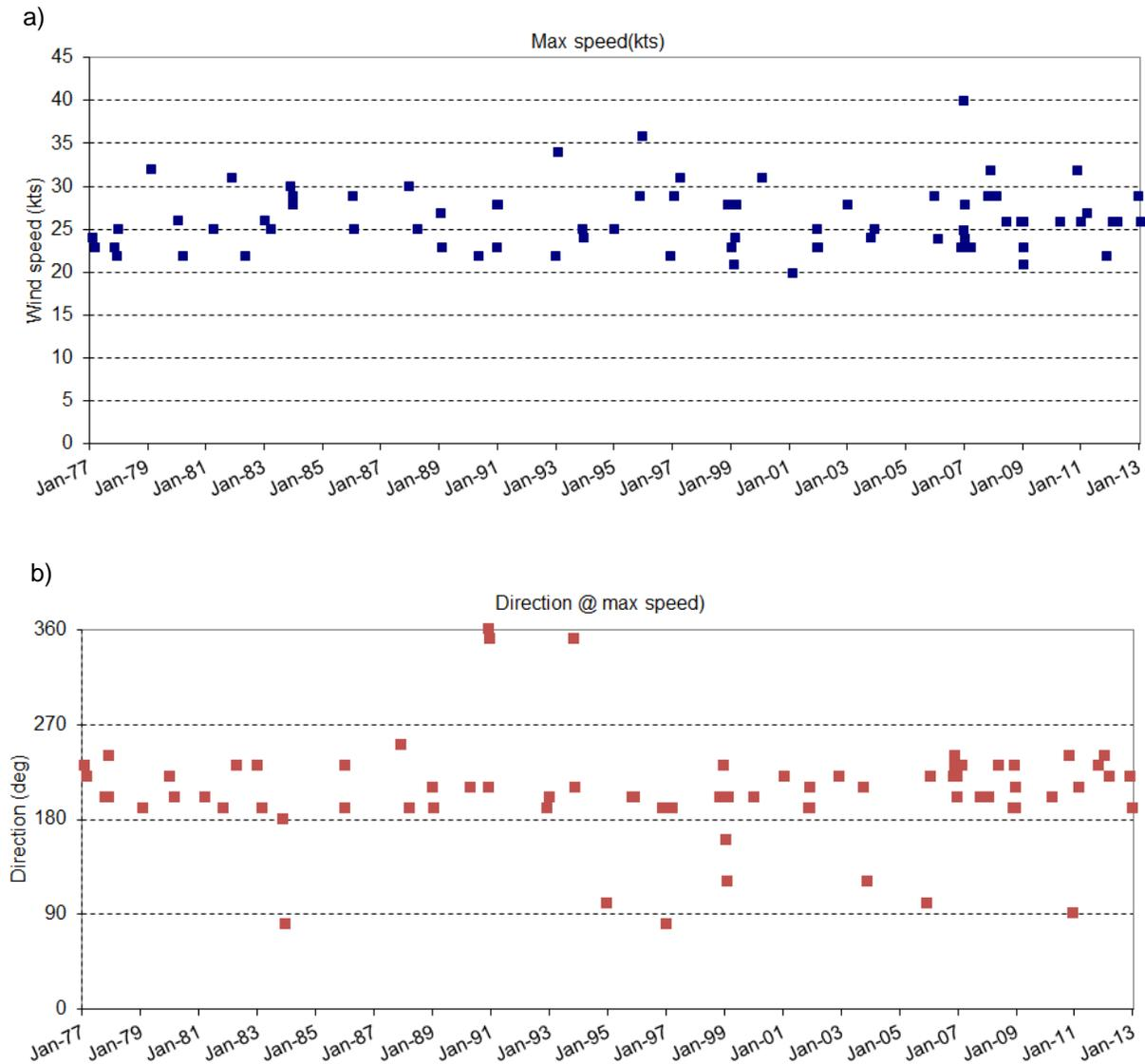
**Figure 2-3: Time series of a) maximum wind speed and b) direction from POT analysis**
