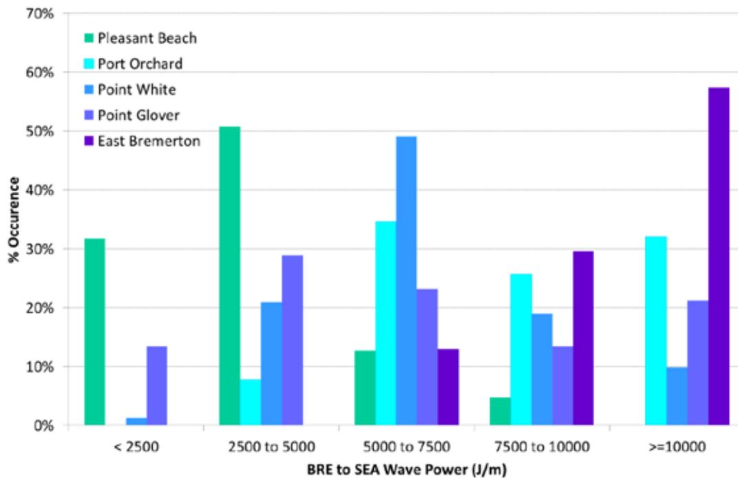
Figure 4-7: Histogram of wave power from RP1 while operating Bremerton to Seattle measured along each shoreline
