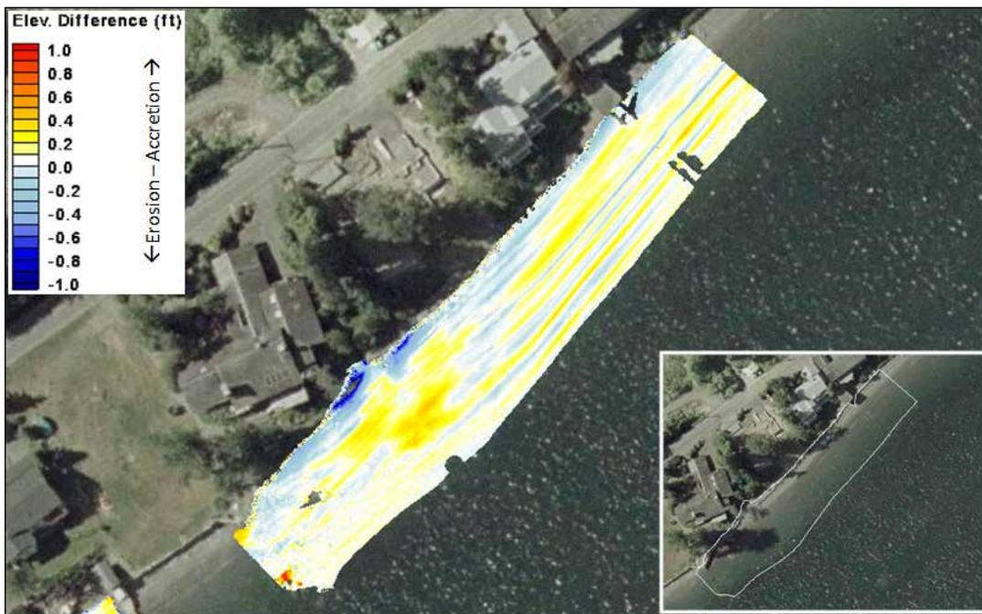
Figure 4-17: Elevation difference at Point White – Site 3 between 12 November and 11 December 2012
