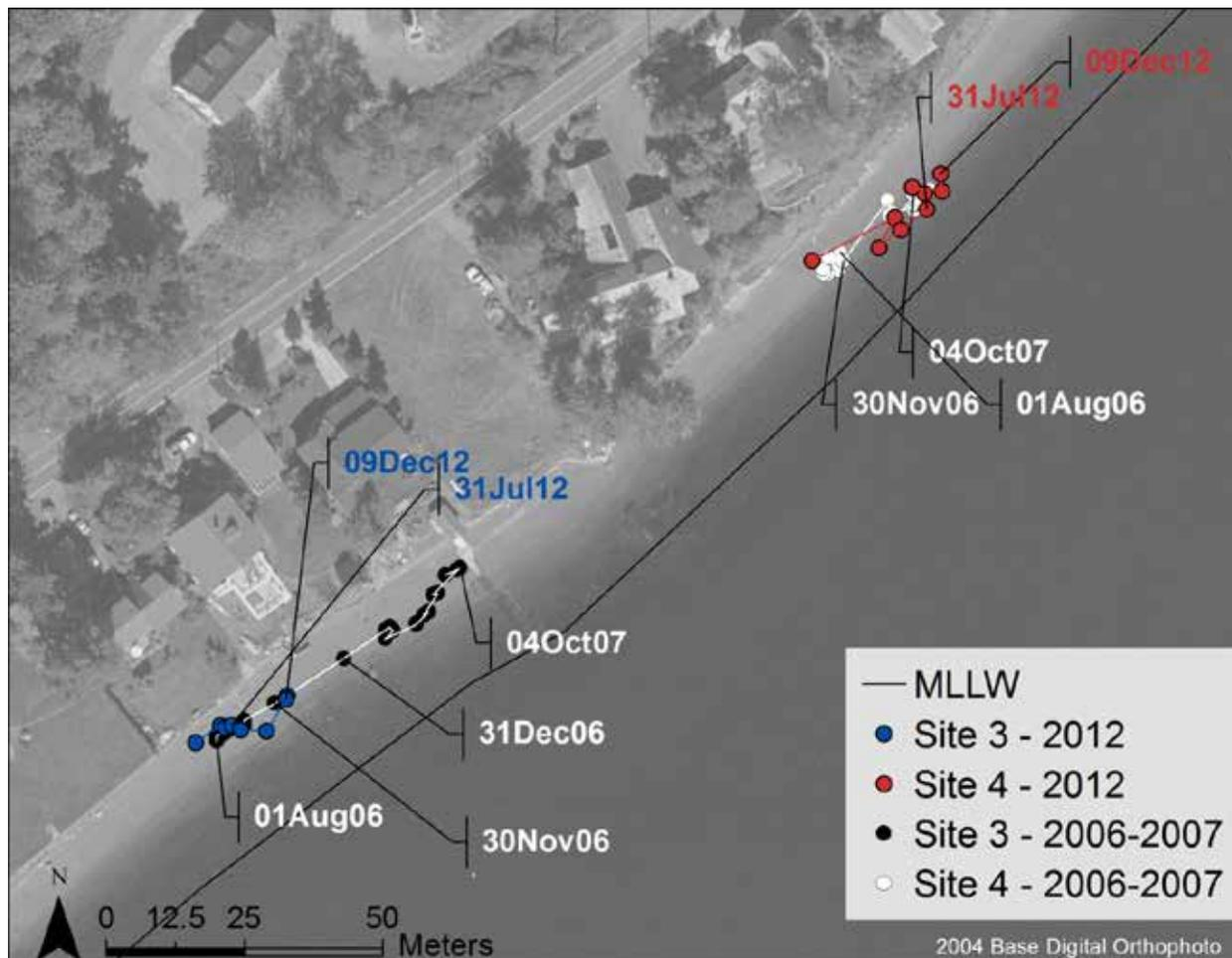
Figure 4-21: Location of tracer centroids for the 2006-2007 and 2012 survey at Sites 3 and 4
